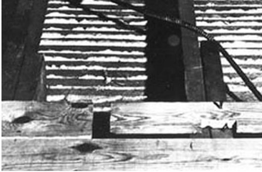
Figure 2. Attic floor above Hauptmann's apartment. with the top left rail of the ladder (right) in place as a continuation of the floor board (left) from which it was fashioned; one nail corresponding to nail hole in the rail and floor joists visible on the rail. With permission of the United States Forest Service.
